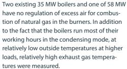
**Optimisation potentials / Weak points:** High flue gas temperature at boiler outlet. Unequal excess air ratio, much higher than optimal.
