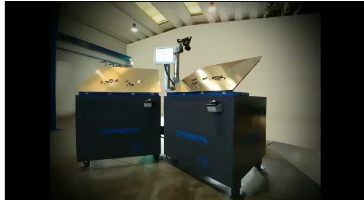
This is an example of a collaborative robotic workstation for wire harnesses assembly that has been designed starting from a manual process to deduce work-related biomechanical overloads.
